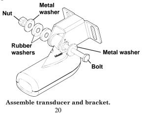
**B.** Two-piece bracket: Once you determine the correct position for the ratchets, assemble the transducer as shown in the figure in step 2B. Don't tighten the lock nut at this time.
